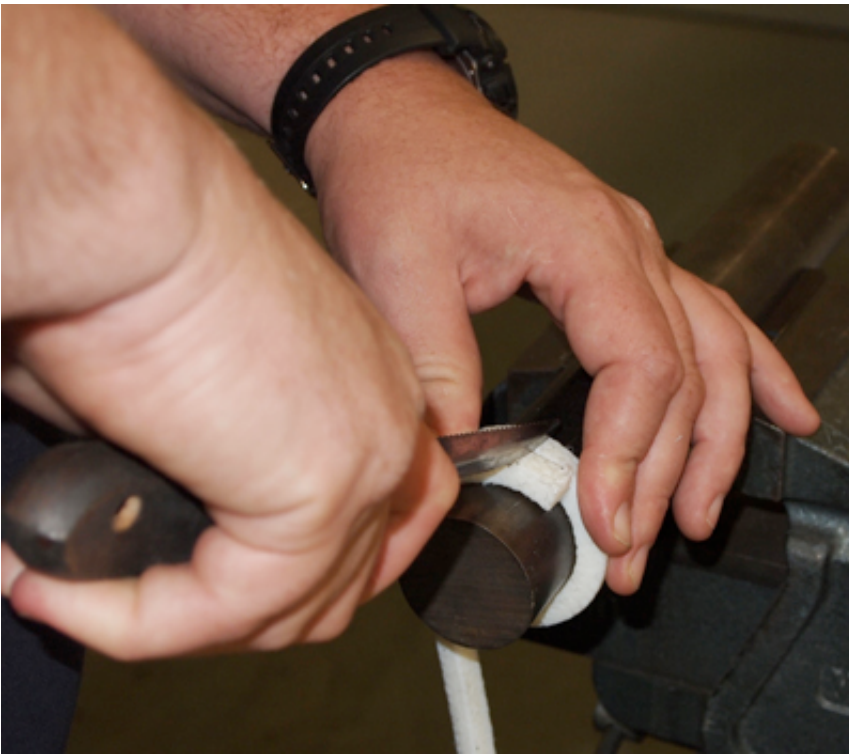
Figure 2. Cutting on a mandrel
